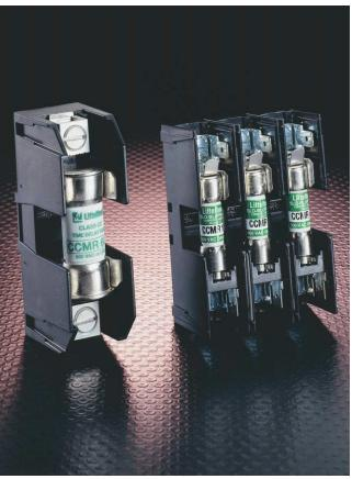
Space-saving 600 volt, 30 amp molded-case fuse blocks with side barriers for isolation. Class CC blocks and Midget blocks are identical except Class CC blocks incorporate a rejection feature to assure proper fusing.
