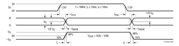
Figure 5. Driver Propagation Delays
