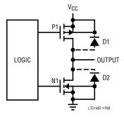
Figure 9. Conventional CMOS Output Stage
