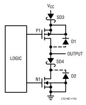
Figure 10. LTC1487 Output Stage
