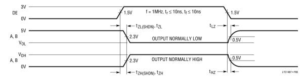
Figure 6. Driver Enable and Disable Times
