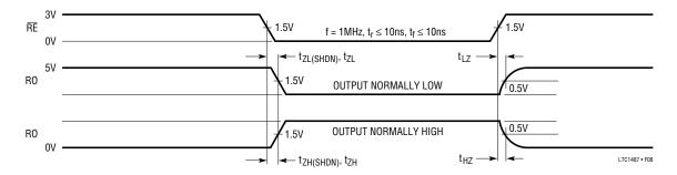
Figure 8. Receiver Enable and Disable Times
