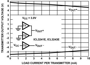
FIGURE 9. TRANSMITTER OUTPUT VOLTAGE vs LOAD
