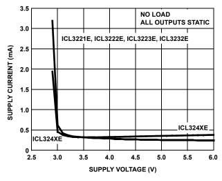
FIGURE 18. SUPPLY CURRENT vs SUPPLY VOLTAGE
