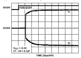
FIGURE 8. TRANSMITTER OUTPUTS WHEN EXITING POWERDOWN
