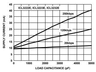
FIGURE 16. SUPPLY CURRENT VS LOAD CAPACITANCE
