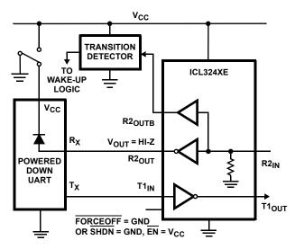
FIGURE 3. DISABLED RECEIVERS PREVENT POWER DRAIN
