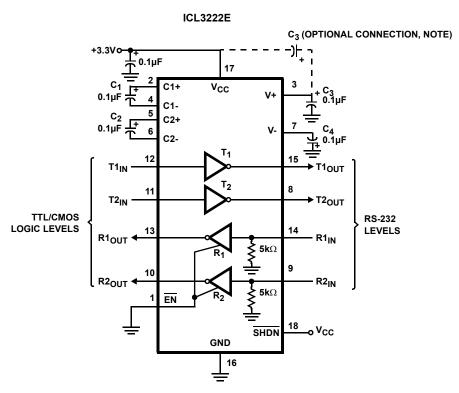
NOTE: The negative terminal of  $C_3$  can be connected to either  $V_{CC}$  or GND
