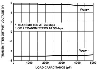
FIGURE 13. TRANSMITTER OUTPUT VOLTAGE vs LOAD
