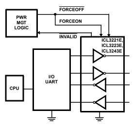
FIGURE 4. CONNECTIONS FOR MANUAL POWERDOWN
