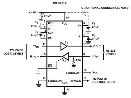
NOTE: The negative terminal of  $C_3$  can be connected to either  $V_{CC}$  or GND
