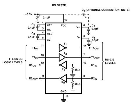
NOTE: The negative terminal of  $C_3$  can be connected to either  $V_{CC}$  or GND
