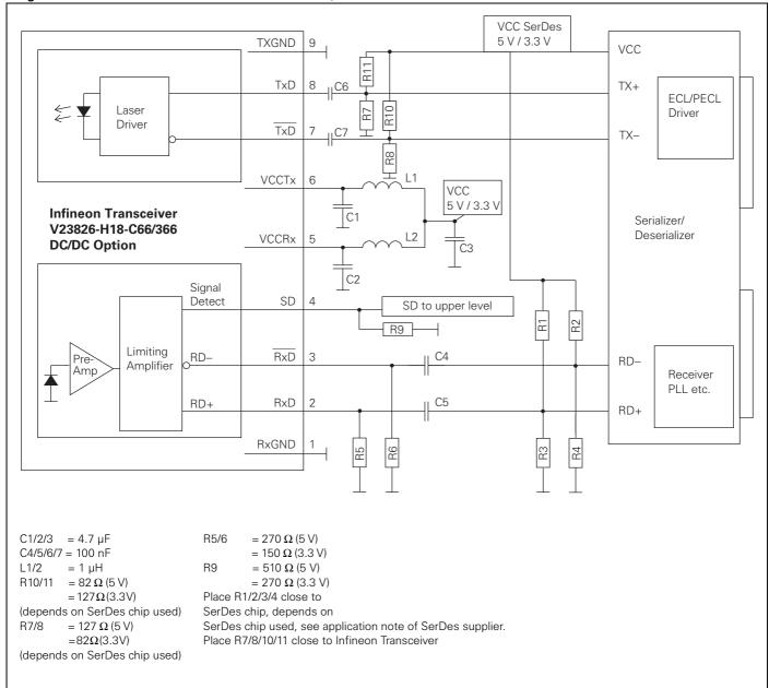
The following Application Notes assume Fiber Optic Transceivers using 5 V power supply and SerDes Chips using 3.3 V power supply. It also assumes no self biasing at the receiver data inputs (RD+/RD-) of the SerDes chip (Refer to the manufacturer data sheet for other applications). 3.3 V-Transceivers can be directly connected to SerDes-Chips using standard PECL Termination network.
