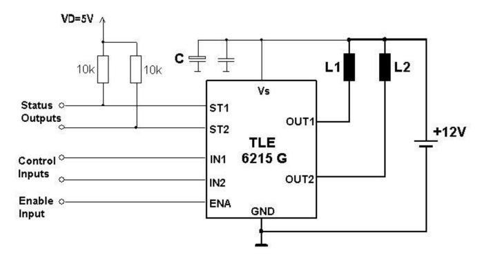
The blocking capacitor C is recommended to avoid critical negative voltage spikes on  $V_{\rm s}$  in case of battery interruption during OFF-commutation.
