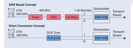
The above figure shows two different tuner concepts for DVB-S/DSS receivers. A satellite dish receives the incoming signal and a LNB converts it to a 1<sup>st</sup> IF signal. In the SAW based concept the 1<sup>st</sup> IF signal is converted to 2<sup>nd</sup> IF by a tuner. Adjacent channels are suppressed by a SAW filter. An I/Q mixer splits up the 2<sup>nd</sup> IF signal into I and Q components and converts the signals to baseband.
