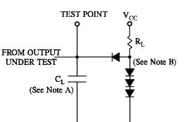
NOTES A. C<sub>L</sub> includes probe and jig capacitance. B. All diodes are 1N916 or 1N3064.
