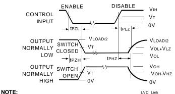
Diagram shown for input Control Enable-LOW and input Control Disable-HIGH.
