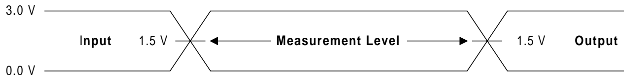
Figure 14. Input Waveforms and Measurement Levels
