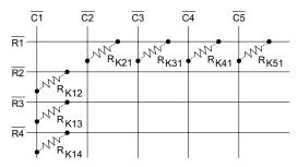
All the resistors are  $330k\Omega$ . The resistor option functions and the default specifications without option resistors are listed below.
