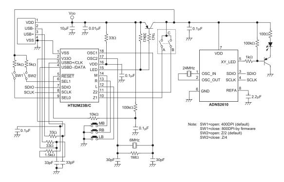
Note: Layout  $0.1\mu F$  capacitor,  $33\Omega$  resistor and  $0.01\mu F$  capacitor as close to VDD pin as possible.
