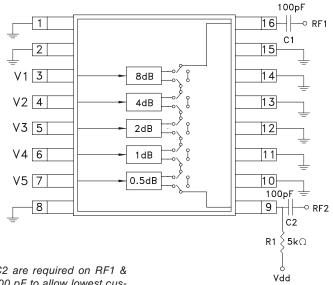
Note: DC Blocking Capacitors C1 & C2 are required on RF1 & RF2. Choose C1 = C2 =  $100 \sim 300 \text{ pF}$  to allow lowest customer specific frequency to pass with minimal loss. R1= 5K Ohm is required to supply voltage to the circuit through either Pin 9 or Pin 16.
