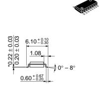
\*Dimension including the plating thickness Base material dimension
