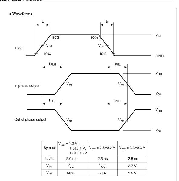
Note: Input waveform: PRR = 10 MHz, duty cycle 50%
