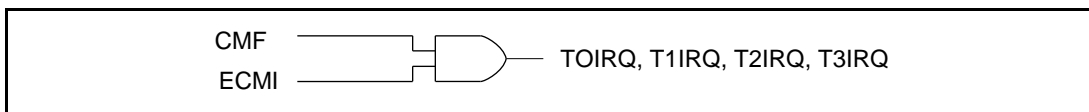
Figure 1.27 Logic Flow for Interrupt Requests, Status, and Enable Bits in Timer Module
