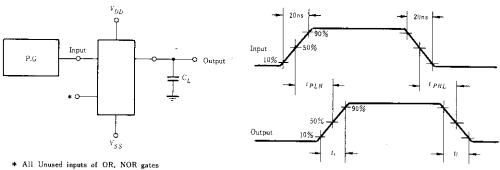
All Unused inputs of OR, NOR must be connected to V<sub>ss</sub>
