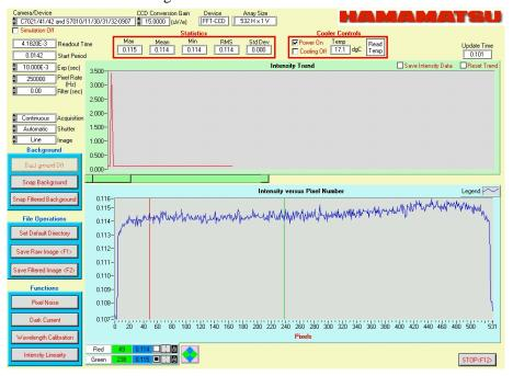
personal computer. The easy of use will enable the end user to focus on the specific application, not computer interface. The new HC230 series includes a cooled camera head, power supply/interface box, LabVIEW drivers and cable assemble. Shown on the right is the main screen of the software. Users can adjust the exposure time, readout frequency, gain and shutter operation. Built
