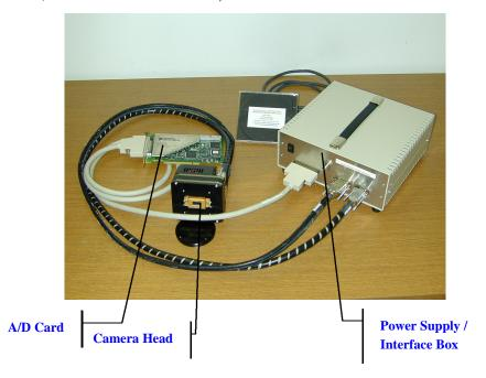
The HC230 series is designed as an OEM evaluation tool. It allows the user to acquire data using a
