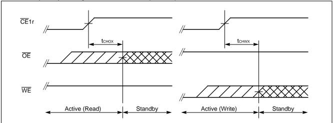
Note: Both tchox and tchwx define the earliest entry timing for Standby mode. If either of timing is not satisfied, it takes trc (Min) period from either last address transition of A<sub>0</sub> and A<sub>1</sub>, or  $\overline{\text{CE}}$ 1r Low to High transition.
