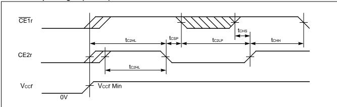
Note: The tc2HL specifies from CE2r Low to High transition after Vccr reaches specified minimum level.
