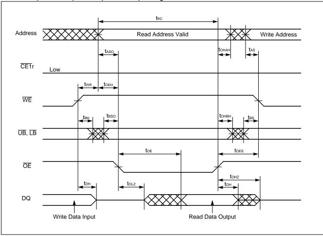
Note :  $\overline{\text{CE1}}$ r can be tied to Low for  $\overline{\text{WE}}$  and  $\overline{\text{OE}}$  controlled operation. When  $\overline{\text{CE1}}$ r is tied to Low, output is exclusively controlled by  $\overline{\text{OE}}$ .
