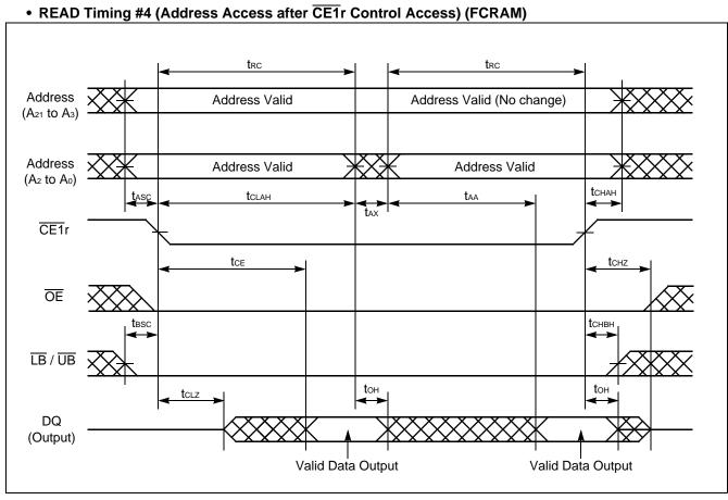
Note: CE2r,  $\overline{\text{PE}}$  and  $\overline{\text{WE}}$  must be High for entire read cycle. Either or both  $\overline{\text{LB}}$  and  $\overline{\text{UB}}$  must be Low when both  $\overline{\text{CE1r}}$  and  $\overline{\text{OE}}$  are Low.
