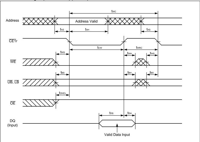
Note: CE2r and  $\overline{PE}$  must be High for write cycle.
