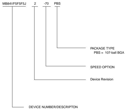
64Mega-bit (4M x 16bit) Dual Operation Flash Memory 64Mega-bit (4M x 16bit) Dual Operation Flash Memory 3.0V-only Read, Program, and Erase
