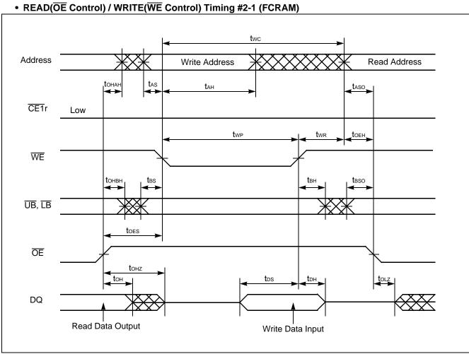
Note :  $\overline{\text{CE1}}\text{r}$  can be tied to Low for  $\overline{\text{WE}}$  and  $\overline{\text{OE}}$  controlled operation. When  $\overline{\text{CE1}}$ r is tied to Low, output is exclusively controlled by  $\overline{\text{OE}}$ .
