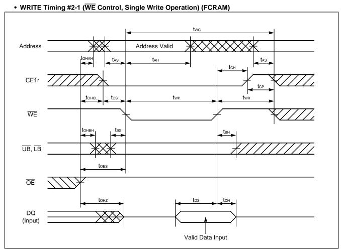
Note: CE2r and PE must be High for write cycle.
