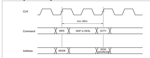
Note: The Mode Register Set command (MRS) should only be asserted after all banks have been precharged and DQ is in High-Z.
