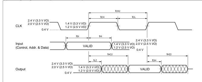
Notes: • Reference level of input signal is 1.4 V for LVCMOS (3.3V I/O),1.2V for LVCMOS (2.5V I/O).
