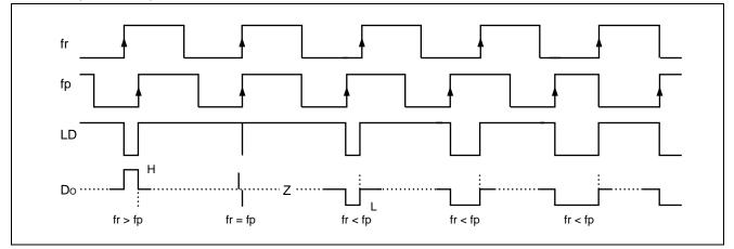
Phase comparator output waveforms are shown below.
