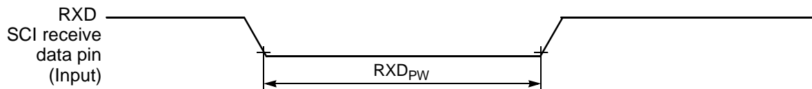
Figure 10-16 RXD Pulse Width
