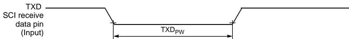
Figure 10-17 TXD Pulse Width
