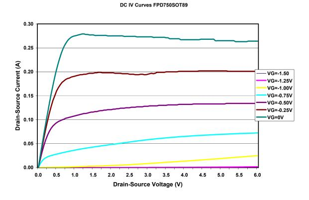
Note: The recommended method for measuring  $I_{DSS}$ , or any particular  $I_{DS}$ , is to set the Drain-Source voltage ( $V_{DS}$ ) at 1.3V. This measurement point avoids the onset of spurious self-oscillation which would normally distort the current measurement (this effect has been filtered from the I-V curves presented above). Setting the  $V_{DS} > 1.3V$  will generally cause errors in the current measurements, even in stabilized circuits.
