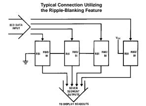
First three stages will blank leading zeros, the fourth stage will not blank zeros.
