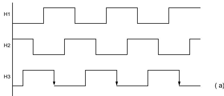
Inversely, if the hall sensors turn on in the order, H3→ H2→ H1, then this shows forward rotation. The output waveforms of the hall sensors are as shown below.
