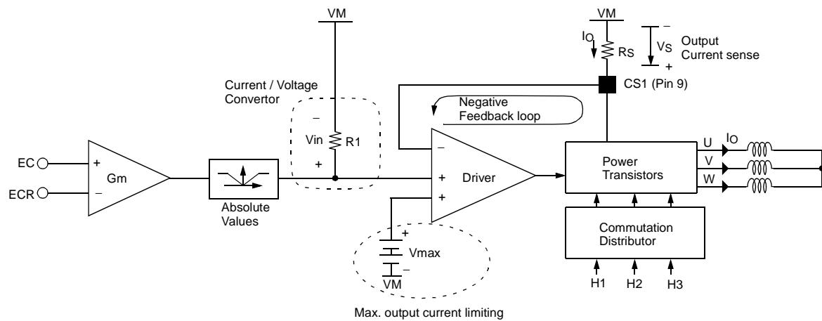
0.255 is made from GM times R1 and is a fixed value within IC.
