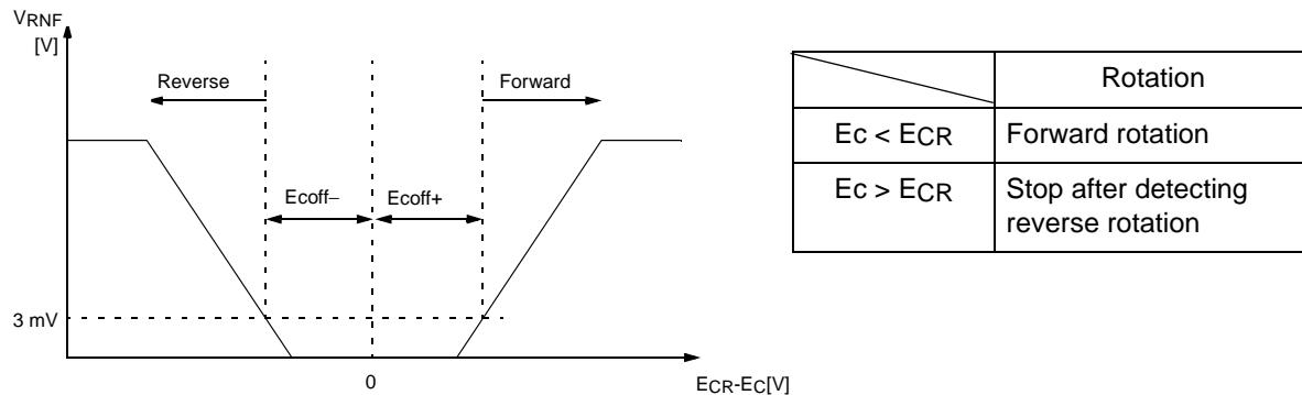
The input range (EC) of the Torque Sense AMP is 0.5V ~ 3.3V
