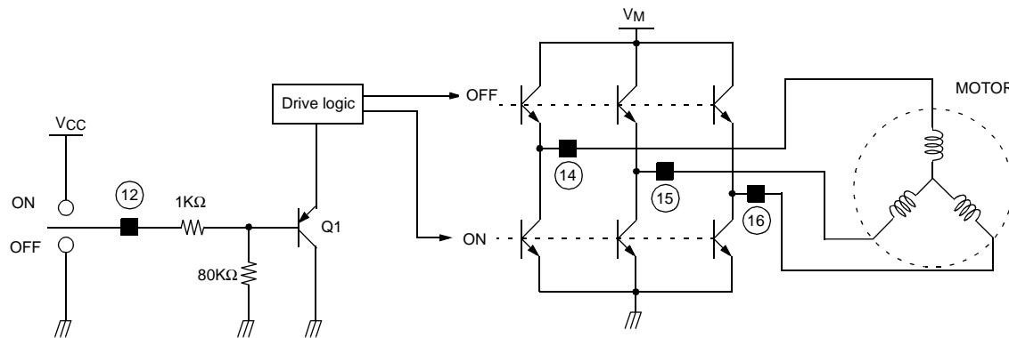
When the pick-up mechanism moves from the inner to the outer spindle of the MD(Mini Disk), the brake function of the reverse voltage is commonly employed to rate the rotational velocity of the spindle motor. However, if the spindle motor rotates rapidly, the brake function of the reverse voltage may produce too much heat at the drive IC.
