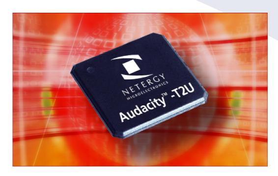
Netergy Microelectronics' Audacity-T2U Voice-over-Packet (VoP) processor is a high performance system-on-a-chip that contains a unified RISC/DSP processor, an Ethernet 10/100 Base-T MAC, and an ATM Utopia interface that is also configurable as a second Ethernet MAC. The Audacity-T2U processor has substantial on-chip SRAM, eliminating the need for external SRAM or DRAM when deployed with Netergy Microelectronics' Veracity VoIP software suite.
