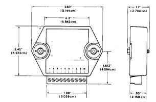
**NOTE**: Spacing for mounting screws = 2.700" (6.858 cm). Screw threads are 6 X 32.
