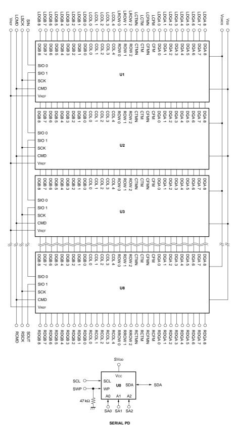
Remarks 1. Rambus Channel signals form a loop through the RIMM module, with the exception of the SIO chain.2. See Serial Presence Detection Specification for information on the SPD device and its contents.
