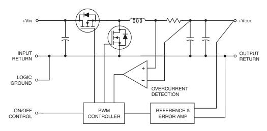
Signals applied to the On/Off Control are referenced to Logic Ground which is internally connected to Input/Output Return. The Logic Ground pin is not designed to carry heavy current. Do not install units with the Return pins open or connected via high-impedance runs.
