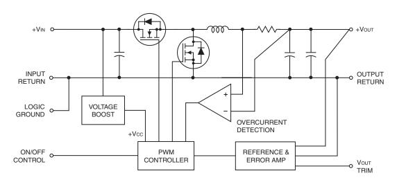
Signals applied to the On/Off Control are referenced to Logic Ground which is internally connected to Input/Output Return. The Logic Ground pin is not designed to carry heavy current. Do not install units with the Return pins open or connected via high-impedance runs.
