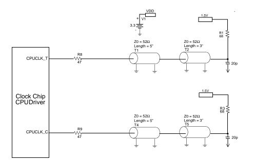
Figure 1. K7 Open Drain Clock Driver Test Circuit
