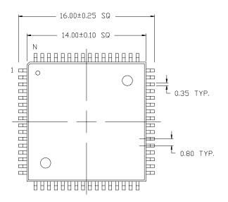
DIMENSIONS IN MILLIMETERS LEAD COPLANARITY 0.102 MAX.
