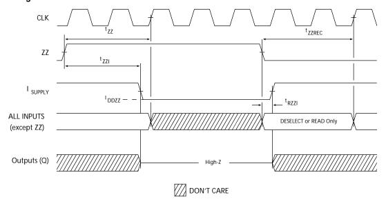
**Notes:**21. Device must be deselected when entering ZZ mode. See truth table for all possible signal conditions to deselect the device.
