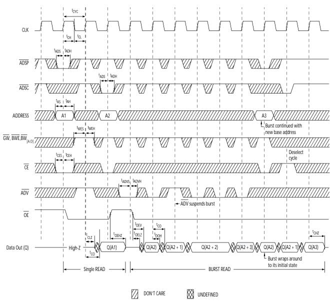
Note: 17. On this diagram, when  $\overline{\text{CE}}$  is LOW:  $\overline{\text{CE}}_1$  is LOW,  $\overline{\text{CE}}_2$  is HIGH and  $\overline{\text{CE}}_3$  is LOW. When  $\overline{\text{CE}}$  is HIGH:  $\overline{\text{CE}}_1$  is HIGH or  $\overline{\text{CE}}_2$  is LOW or  $\overline{\text{CE}}_3$  is HIGH.
