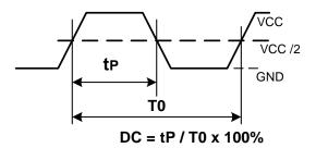
Figure 4. Output Duty Cycle (FoutDC)
