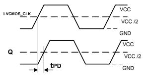
Figure 3. LVCMOS Propagation Delay (TPD) Test Reference
