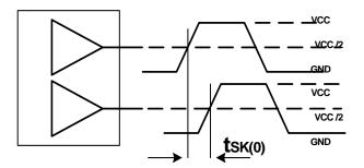
Figure 5. Output-to-Output Skew tsk(0).
