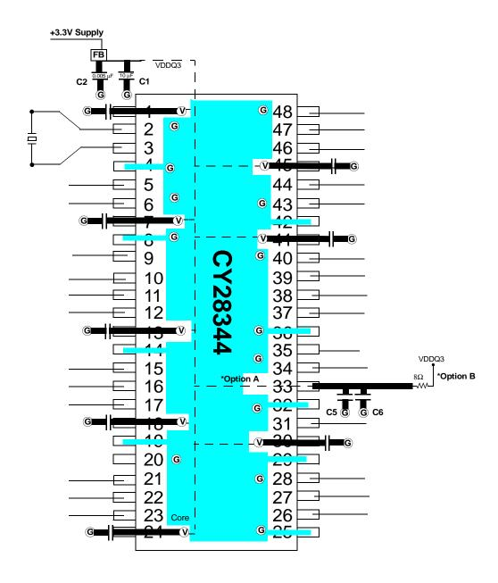
FB = Dale ILB1206 - 300 or 2TDKACB2012L - 120 or 2 Murata BLM21B601S Ceramic Caps C1 = 10 - 22  $\mu F$  C2 = 0.005  $\mu F$  C5 = 0.1  $\mu F$  C6 = 10  $\mu F$  ©= VIA to GND plane layer( $\hat{V}$ = VIA to respective supply plane layer Note. Each supply plane or strip should have a ferrite bead and capacitors.
