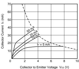
COLLECTOR CURRENT vs. **COLLECTOR SATURATION VOLTAGE**
