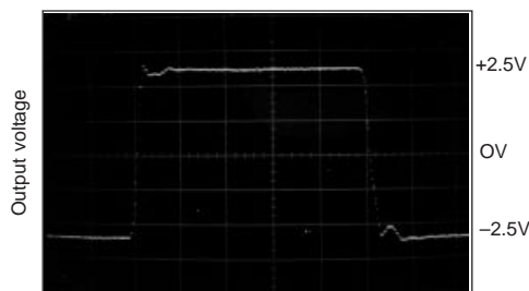
Output Voltage - 5Vp-p, 5ns/DIV
