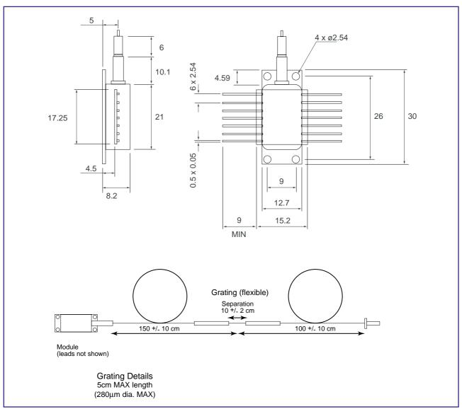
Figure 1: Package Outline Drawing and Dimensions (mm)
