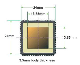
The form factor of the AF-S2 is 68-pin JEDEC-standard Plastic Leadless Chip Carrier (PLCC).
