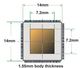
The form factor of the EntréPad AES3400 is 100-pin JEDEC-standard Low-profile Quad Flat Package (LQFP)
