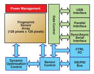
The EntréPad AES3400 sensor incorporates flexible SelectaBus architecture. This feature allows the developer to deploy designs that use not only the popular Universal Serial Bus, but also synchronous and asynchronous serial interfaces, and an 8-bit parallel interface implementation.
