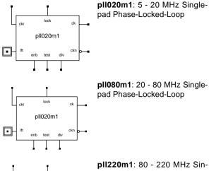
pll080m1: 20 - 80 MHz Singlepad Phase-Locked-Loop
