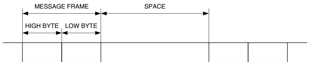
Figure 7. Message Frame and Space
