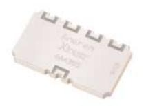
The 4A3305 is a low profile 4 way Wilkinson power divider in an easy to use surface mount package designed for DCS, PCS, UMTS, W-LAN and other 3G applications. The 4A4305 is ideal for low power, In-Phase divider/combiner applications. Parts have been run through rigorous qualification testing and units are 100% tested. They are manufactured using materials with x and y thermal expansion coefficients compatible with common substrates.
