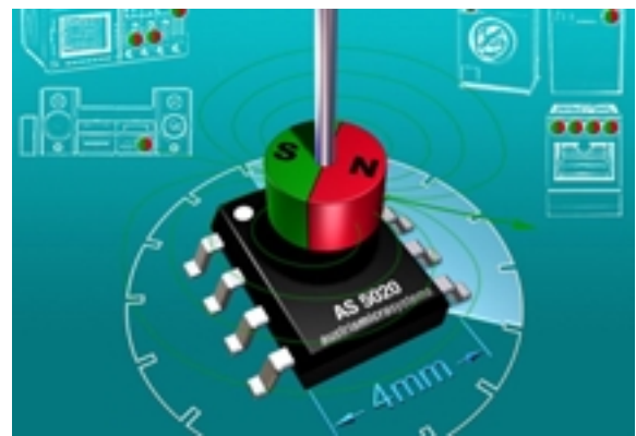
Figure 1 Placement of AS5020 device and magnet source
