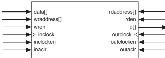
Figure 7-4. Simple Dual-Port Memory Note (1)
