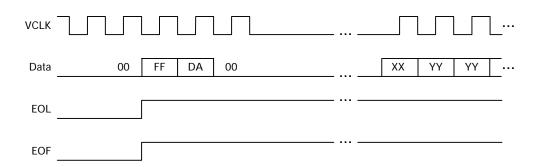
The ADCC-3960 does not generate a full JFIF header for JPEG data. The FF DA 00 XX four byte header specifies which Q table was used to compress the data. See the *ADCC-3960 SXGA CMOS Imager Register Reference* for details on how to use this information to create the JFIF header.
