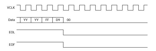
The FF D9 is the valid end of image indicator. There are many other options for the JPEG output (see ADCC-3960 SXGA CMOS Imager Register Reference for additional information).
