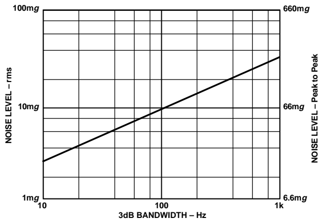
Figure 19. ADXL150/ADXL250 Noise Level vs. 3 dB Bandwidth (Using a “Brickwall” Filter)
