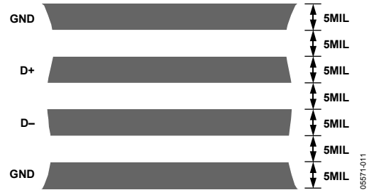
Figure 23. Typical Arrangement of Signal Tracks
