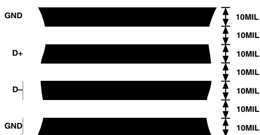
Figure 6. Arrangement of Signal Tracks
