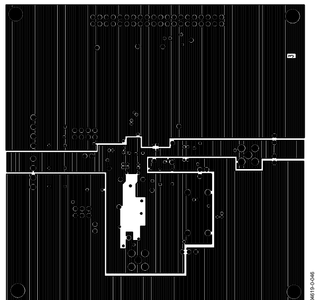
Figure 46. PCB Split Power Plane
